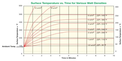
△T = Temperature Rise From Ambient at Specified Watt Densities
